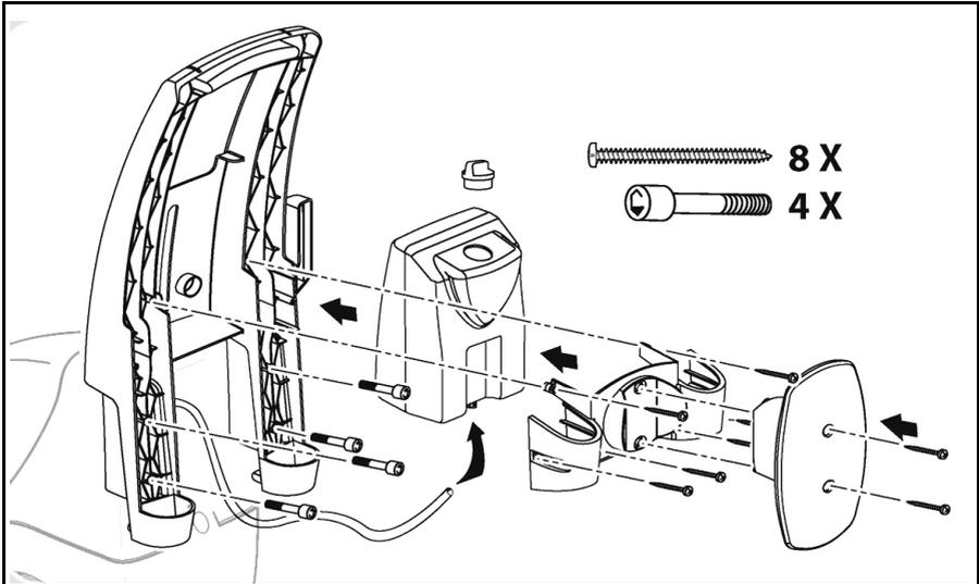
1. Fit the handle first then the detergent tank, followed by the tool holder and finally the hose hook to the hot washer as shown above using the 4 bolts (for the handle) and screws (for the tool holder, hose hook) supplied.
