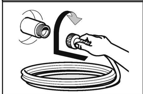
6. Screw the high pressure hose onto the gun assembly.
