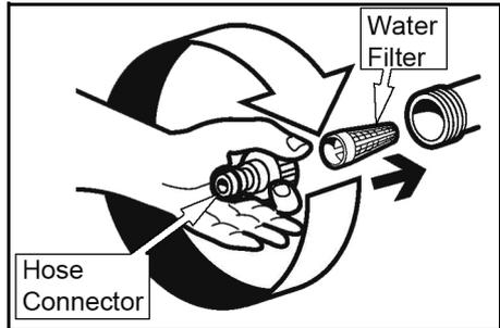
4. Connect the water supply hose to the hose connector. The hose must have an inside diameter of at least 13 mm (1/2").
